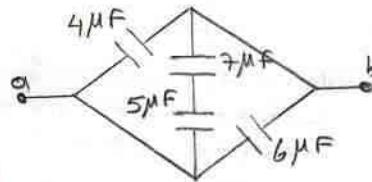
$$\text{Cevap: } C_s = \left( \frac{1}{5} + \frac{1}{7} \right)^{-1} = 2,92\mu\text{F}$$
